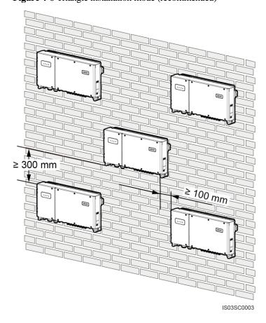
Figure 4-6 Triangle installation mode (recommended)
