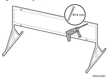
Step 4 Align the mounting bracket with the hole positions, insert bolt assemblies (flat washers, spring washers, and M12x40 bolts) into the holes through the mounting bracket, secure them using the shipped stainless steel nuts and flat washers, and tighten the bolts to a torque of 45 N·m using an 18 mm socket wrench.
