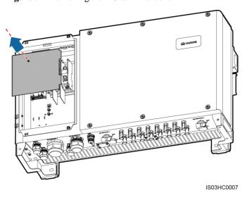
Figure 5-7 Removing the AC terminal cover
