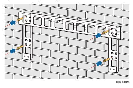
Figure 4-14 Securing a mounting bracket
