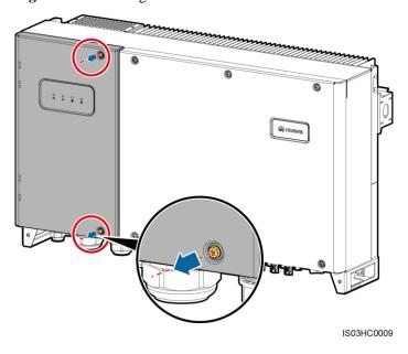
**Step 2** Open the maintenance compartment door and install a support bar.
