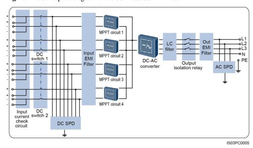
Figure 2-10 Conceptual diagram for the SUN2000-33KTL-A/36KTL
