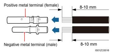
**Step 2** Insert the exposed area of the positive and negative power cables into the metal terminals of the positive and negative connectors respectively and crimp them using a crimping tool, as shown in Figure 5-19. Ensure that the cables are crimped tightly such that they cannot be pulled out by a force less than 400 N.
