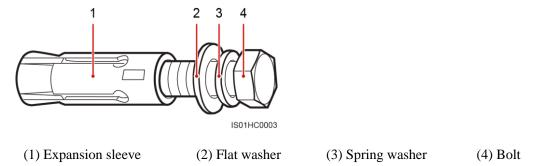
Figure 4-13 Drilling a hole and installing an expansion bolt
