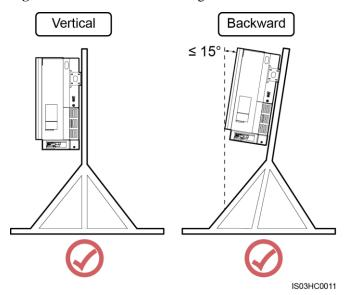
• Do not install the SUN2000 at a front tilt, excessive back tilt, side tilt, horizontally, or upside down.
