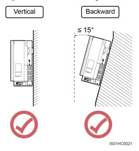
Do not install the SUN2000 at a front tilt, excessive back tilt, side tilt, horizontally, or upside down.
