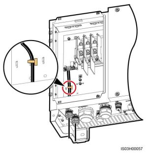
**Step 8** Use a torque wrench with an open end of 33 mm to tighten the locking cap to a torque of 7.5 N•m.
