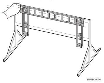
Figure 4-24 Determining hole positions
