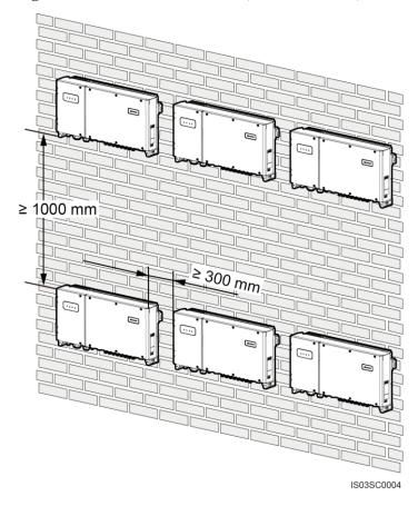
Figure 4-7 Stacked installation mode (not recommended)
