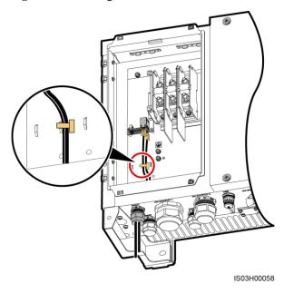
Figure 5-35 Binding communications cables
