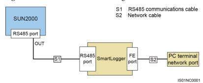
Figure 5-26 shows the communication mode for multiple SUN2000s.
