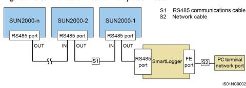
Figure 5-26 Communication mode for multiple SUN2000s
