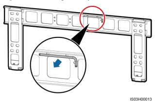
**Step 2** Determine the positions for drilling holes using the mounting bracket. Level the hole positions using a level, and mark the hole positions using a marker.
